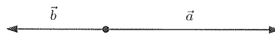
Figure 10.33: Vectors \vec{a} and \vec{b} in opposite direction: max \|\vec{a} - \vec{b}\| , min \|\vec{a} + \vec{b}\|
